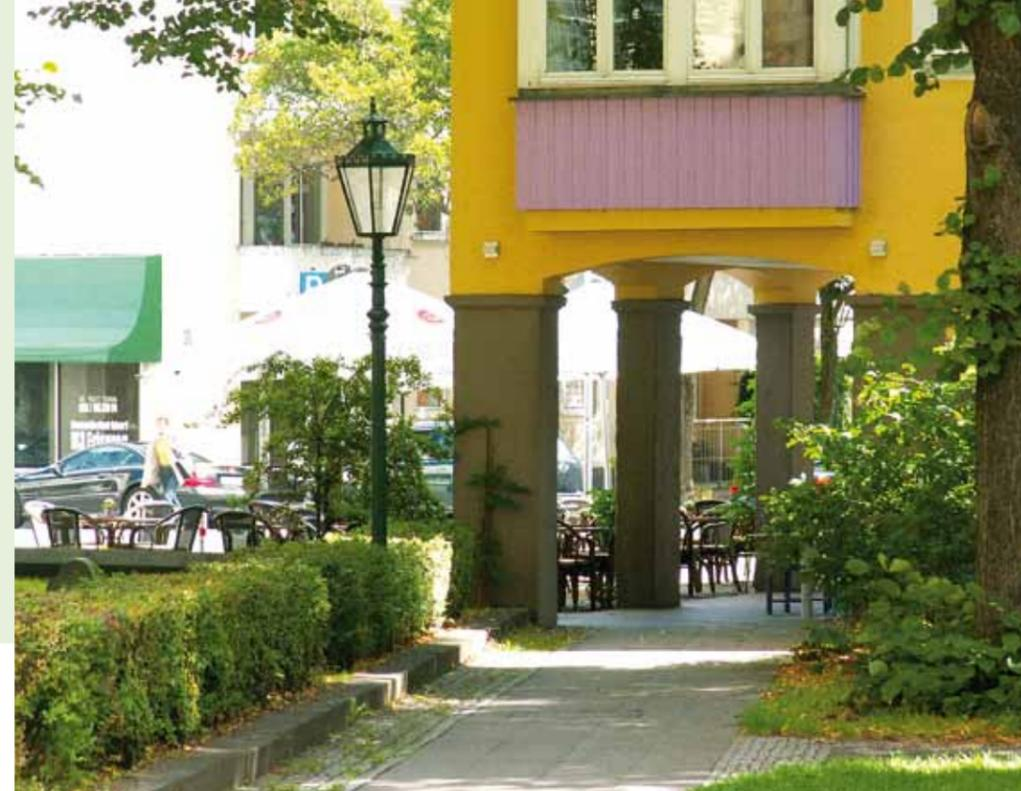
Figure 25: Sun protection through arcade (centre), sunshades (background) and sun shield (left edge, middle)
