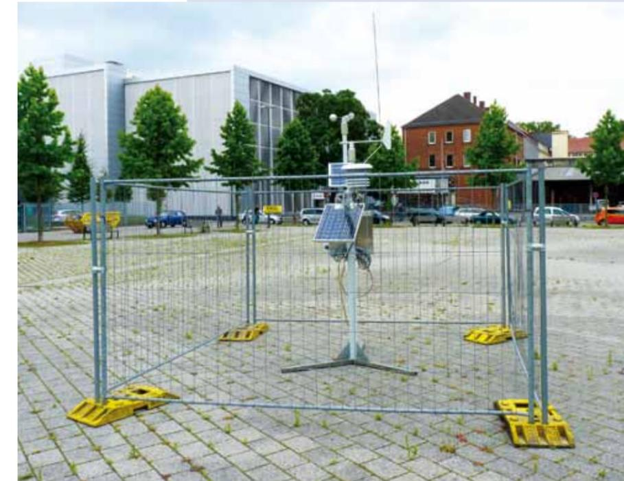
Figure 32: Mobile climate monitoring station of the German Meteorological Service in Bremen (Photo: DWD)
